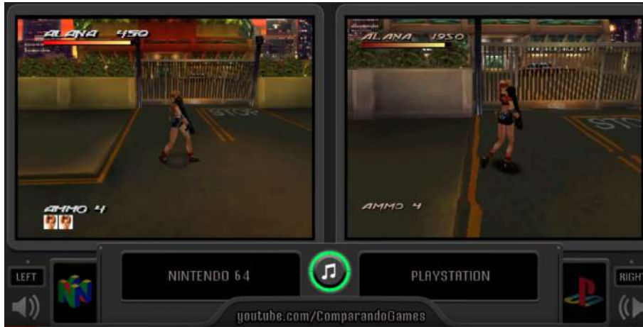
Fig. 5. PlayStation1 (right) didn't have correct texture mapping due to absence of floating point for pixel operations [19].
