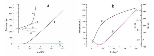
Figure 2: Maximum values of the total pressure (1), its thermoacoustic component (positive 2 and negative 3), surface temperature (4), and surface displacement value  $\Delta z$  at t = 200 ns (5) versus laser fluences.
