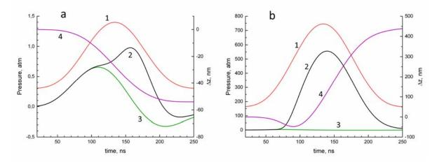
Figure 1: Time dependence of thermoacoustic pressure part (3), total (including vaporization) pressure (2) and irradiated surface displacement  $\Delta z$  (4) during laser pulse (1) action at different fluences E = 20 (a) and 200 (b) mJ/cm<sup>2</sup>.
