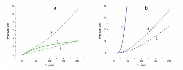
Figure 6: Maximum values of the pressure component: smooth (1) and modulated (2, 3), thermoacoustic (a) and vaporisation (b) versus laser fluence E.
