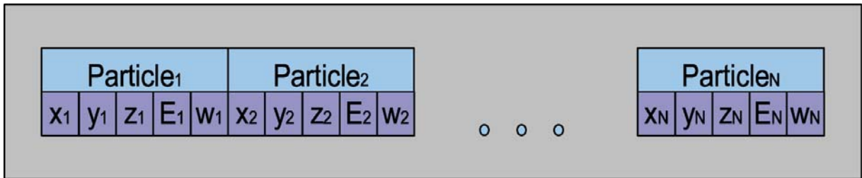
Figure. 1 – optimal data storage layout for CPU.
