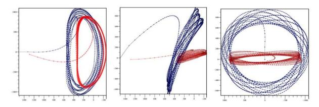
Fig. 4. 2D view of the quasi periodic orbits, proposed for "Spectr-RG" (red) and "Millimetron" (blue) spacecraft in the rotating  $L_2$  centered reference frame (X-axis points from the Sun)
