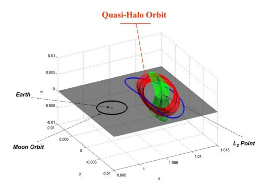
Fig.1. Periodic and quasi periodic orbits in the vicinity of the  $L_2$  point. Blue color represents planar and vertical Lyapunov orbits, black color – halo orbit with red quasi periodic orbit around it, green color – Lissajous orbit.
