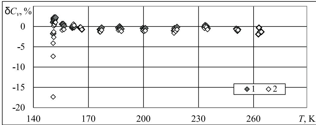
Figure 4: Relative deviations \delta C_V = (C_{V,\text{exp}} - C_{V,\text{cal}})/C_{V,\text{exp}}100\% ; p_{\text{cal}} : C_{V,\text{cal}} corresponded to values calculated with the help of (1) in the single phase range; C_{V,\text{exp}} corresponded to data [48] over isochoric line 473.6 \text{ kg/m}^3 ; 1— C_V calculated with the help of FEOs (1); C_V calculated with the help of FEOs [9].
